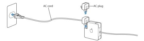
*Warning:* Make sure the power adapter is fully assembled before plugging it into an electrical outlet. If you're using the AC plug with your power adapter, make sure the two prongs are snapped into their completely extended position before plugging in the adapter.
