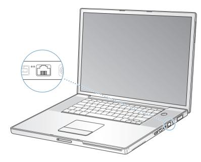
Connecting to a network gives you access to other computers. You may be able to store and retrieve information; use network printers, modems, and email; or connect to the Internet. You can also use Ethernet to share files between two computers or set up a small network. The Ethernet port on your PowerBook automatically detects other Ethernet devices. You don't need an Ethernet crossover cable when connecting to other Ethernet devices.
