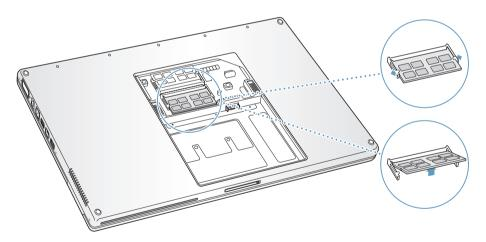
6 Insert the memory card at a 30-degree angle. Line up the notch in the card with the small tab in the memory slot and slide the card into the slot until the gold edge is almost invisible. Then gently push the memory card into the memory slot. You may feel some resistance.
