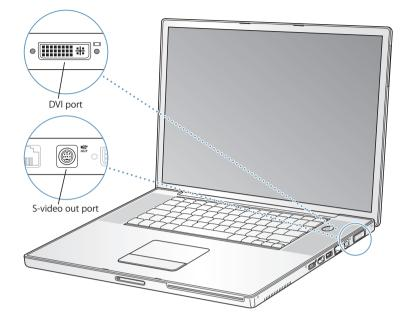
When an external monitor or television is connected, you can either have the same image appear on both the internal display and the external monitor (known as *video-mirroring*) or use the external monitor to extend the size of the Mac OS desktop (known as *dual-display mode*). By default, your PowerBook starts up in dual-display mode. Press the F7 (日) key to switch between dual-display and video-mirroring modes.
