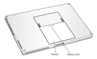
If the battery icon in the Finder menu bar is set to show the percentage of charge, you may sometimes notice that the battery does not maintain a full charge of 100 percent when the power adapter is attached. When the battery level eventually drops below 95 percent, it will charge all the way to 100 percent. This saves battery life as charging is not continuously cycled on and off.
