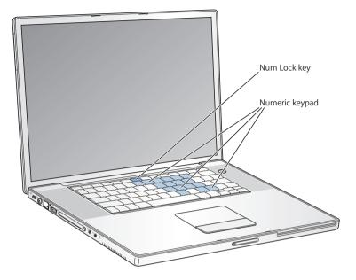
To use the numeric keypad, press the Num Lock key. The Num Lock key glows green, indicating that the keypad is active. When you're finished, press the Num Lock key again to turn it off.
