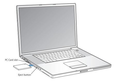
*Important:* The Apple AirPort Extreme Card is installed in a slot inside the computer. It doesn't go in the PC Card slot the way many third-party wireless cards do. The AirPort Extreme Card will not work if it is installed in the PC Card slot and will cause your computer to function improperly.
