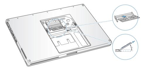
7 Gently spread the small tabs in the memory slot away from the notches and push the memory card down until the two snaps on either side of the card lock into place.
