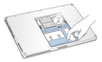
5 If you already have a memory card installed in the slot you wish to use, remove it. Spread the tabs in the slot away from the notches in the memory card. The card should pop up slightly. Lift the memory card to a 30-degree angle and then gently slide the card out of the memory slot.
