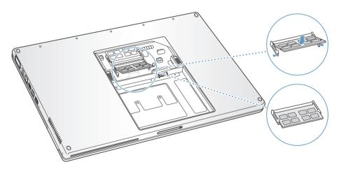
8 Replace the memory door and make sure it is lying flat before screwing it into place.
