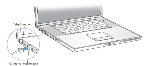
Make sure you connect the internal modem to an analog phone line—the kind used typically in homes. The modem will not work with a digital phone line.
