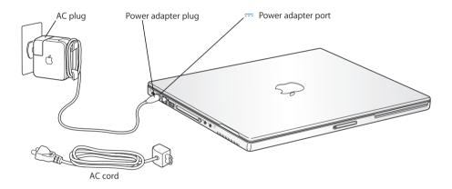
To extend the reach of your power adapter, you can attach the AC cord if desired. See "Using Your Power Adapter" on page 23.
