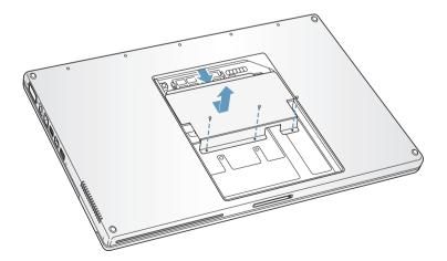
4 Touch a metal surface inside the computer to discharge any static electricity from your body.
