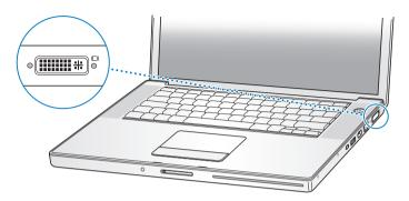
When an external monitor or TV is connected, you can either have the same image appear on both the built-in display and the external monitor (known as *video mirroring*) or use the external monitor to extend the size of the Mac OS desktop (known as *dual-display* or *extended desktop mode*). By default, your MacBook Pro starts up in dual-display mode. Press the F7 (日) key to switch between dual-display and video-mirroring modes.
