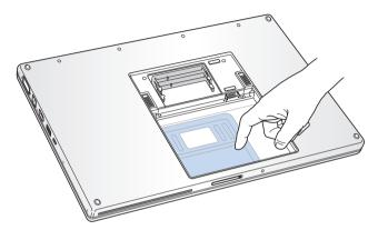
3 If you already have a memory card installed in the slot, remove it. Spread the tabs in the slot away from the notches in the memory card. The card should pop up slightly. Lift the memory card to a 25-degree angle and then gently slide the card out of the memory slot.
