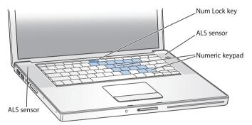
To use the numeric keypad, press the Num Lock key. The Num Lock key glows green, indicating that the keypad is active. When you finish using the keypad, press the Num Lock key again to turn it off.
