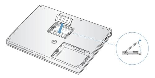
5 Press down on the memory card to lock it in place. If the memory card does not latch, do not force the card down. Try reinserting the card to make sure it is fully seated.
