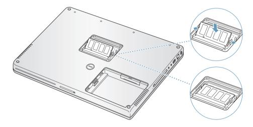
6 Replace the memory door and screw it in place.
