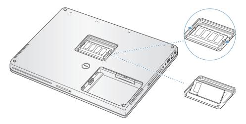
4 Insert the new memory card into the slot at a 30-degree angle. Push the card to seat it fully in the slot.
