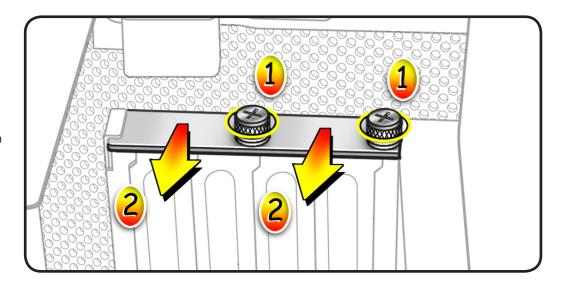
**Note:** If card is held in place by retention bar, complete steps 4 and 5. Otherwise, release small locking clip at front of card's connector by pushing clip up. Then go to step 6.
