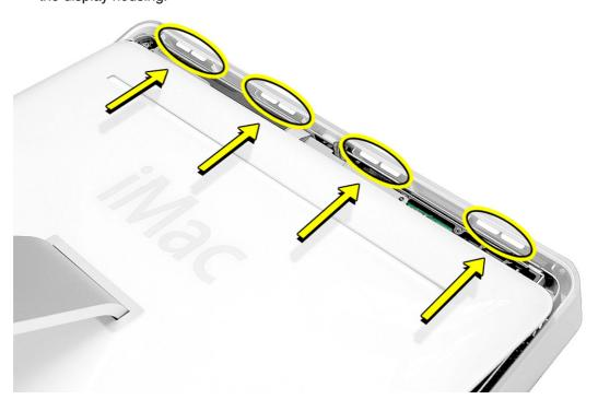
2. Tilt the back cover slightly and align the top edge with the tabs on the housing. Push the two together as you lower the back cover.
