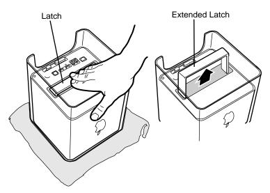
7 Gently pull the core from the computer enclosure and place the core on a soft cloth.
