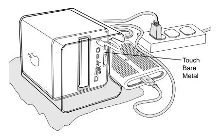
**Important:** To avoid electrostatic discharge, always ground yourself by touching the bare metal before you touch any parts or install any components inside the computer. To avoid static electricity building back up in your body, do not walk around the room until you have completed the installation and closed the computer.
