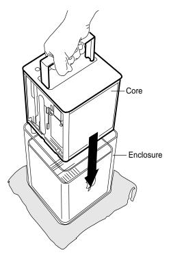
2 With a flat hand, press down on the latch until it locks into place. Firmly press the core to ensure it is fully secured within the enclosure.
