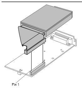
Installing an Internal IDE Hard Disk
