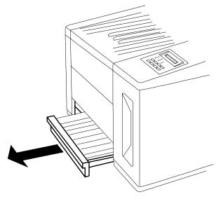
2 On the envelope cassette, open the stacker arm and set the side and rear envelope stackers to the correct envelope size.
