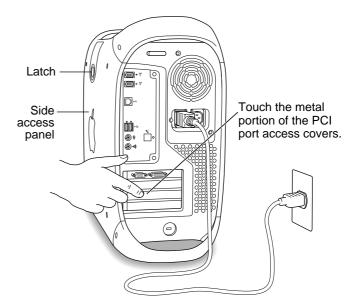
**Important:** To avoid electrostatic discharge, always ground yourself by touching the port access covers before you touch any parts or install any components inside the computer. To avoid static electricity building back up in your body, do not walk around the room until you have completed your installation and closed the computer.
