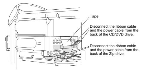
6 Slide the drive carrier assembly the rest of the way out of the computer.
