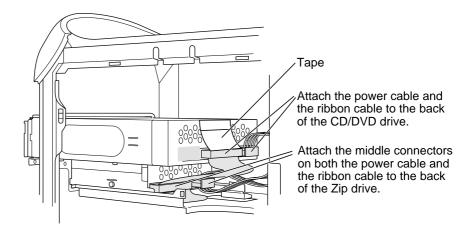
5 Push the drive carrier the rest of the way into the computer.
