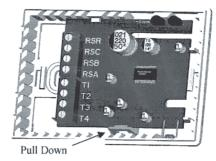
5. Use the subbase as a template to mark the mounting hole locations on the wall. The word "TOP" will be written in the subbase. Position the subbase so that the wires can be pulled through the hole in the top left-hand corner. Drill size for the wall anchors is 3/16 inch. Mount the subbase using the two #6 screws and anchors provided (larger screws will prevent the circuit board from properly snapping into place).
