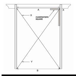
When the arbor is square, drive the second screws into the posts securing them to the header.
