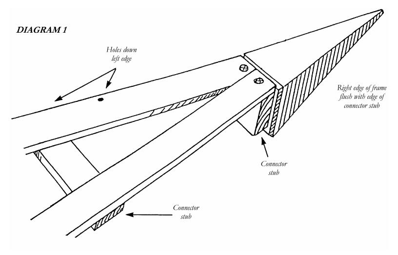
Holding the trellis end firmly against the base of the pyramid cap and with its right edge flush to the connector stub, drive in the right-hand screw. Then drive in the left screw, again keeping a snug fit.
