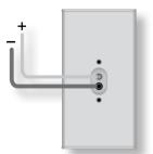
Refer to your amplifier/receiver/sound processor handbook to identify the speaker terminals and their polarity. For each speaker, connect the positive terminal of the amplifier (normally coloured red or labelled with '+') to the red (positive) terminals on Muso. Similarly, connect the negative terminal of the amplifier (normally coloured black or labelled with '-') to the black (negative) terminals on Muso.
