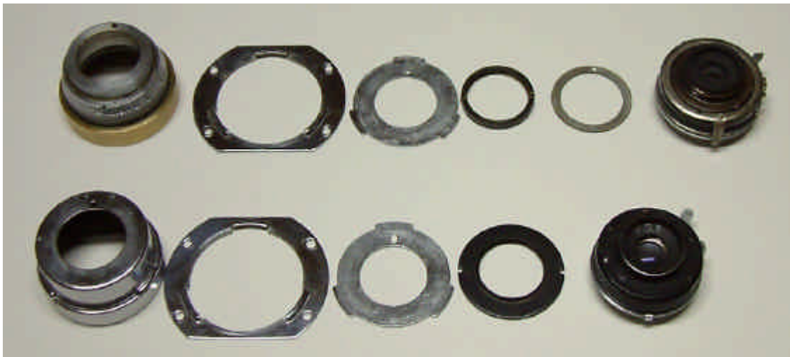
Fig. 7-3: Two separated Neck and Shutter assemblies; AF (top) and post-war A2B (bottom)
