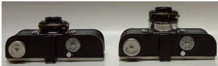
Fig 5-2: The Neck and Shutter in the storage position (left), and the extended position (right)
