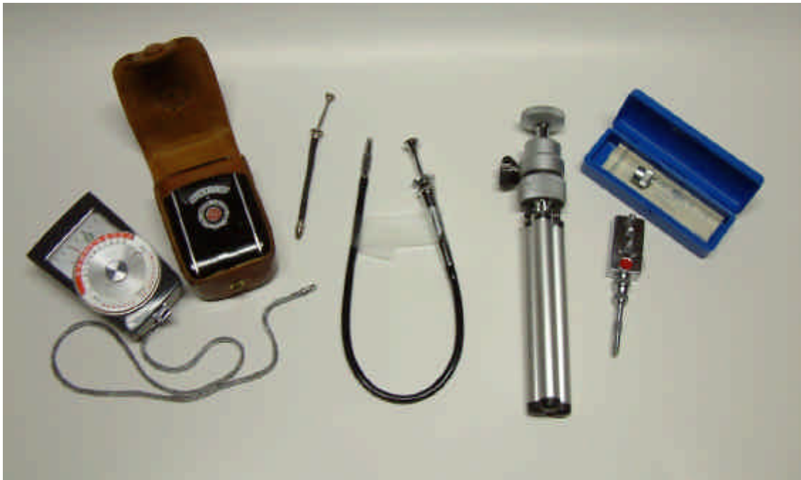
Fig. 6-3: (From left to right) Two light meters, two cable releases, a tripod, and a self-timer.
