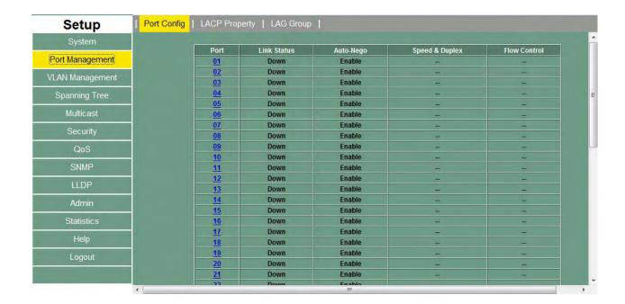
**Port Management – Port Config - Specific Port.** Settings can be made on a per port basis. When a port number is clicked the subscreen appears.
