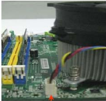
Cooler power cable
