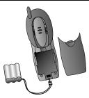
b) Plug the battery pack connector into handset.Place the battery pack and wires in the compartment.
