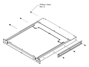
2. Attach the left and right *easy-installation* mounting rails to the inside of the rack. The flange that supports the switch will be to the inside.
