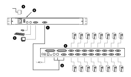
**Note:** The example diagram shows the CL-1200 connecting to an ACS-1216A KVM switch, but the CL-1200 can connect to most ATEN KVM switches that have PS/2 port console connectors. If you are connecting to a different model, the console port connectors may be in a different location.
