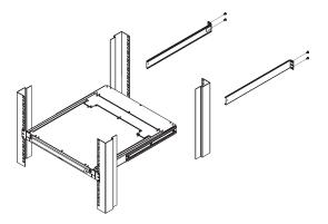
3. After the L brackets have been secured, tighten the front bracket screws
