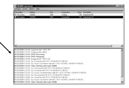
Note that even though any other CN-5000s aren't currently selected, if their *Recording* checkbox is checked, the Log Server records their tick information and keeps it in its database. You can see the server's tick information by selecting it.
