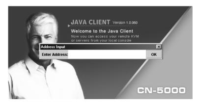
4. Key in the IP address for the unit you want to connect to - including a forward slash followed by the name of the CN-5000's Default Java Program Name (see p. 19). For example:
