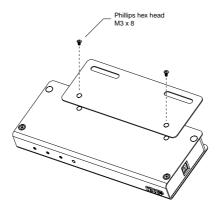
2. Screw the bracket into any convenient location on the rack.
