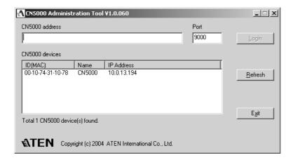
The DHCP assigned IP address appears in the right hand column of the *CN5000 Devices* panel:
