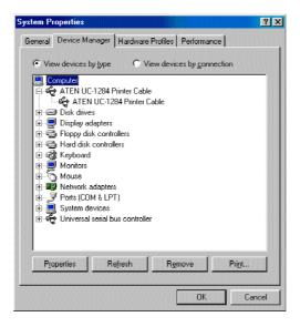
Now double click on ATEN UC-1284 Printer Cable (UC1284USBx). If the installation was successful, an ATEN UC-1284 Printer Cable Properties box will appear and the device status will state that the device is working properly.
