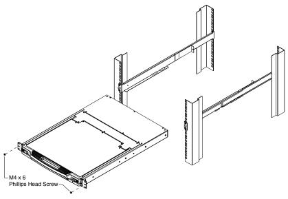
4. Slide the rear attachment sliding brackets along the slide bars until they contact the rear of the switch, then use the screws supplied with this package to attach the bars to the rear of the switch (tighten the screws all the way).
