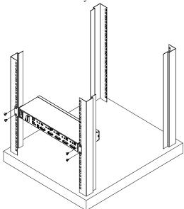
**Note:** These screws are not provided. We recommend that you use M5 x 12 Phillips Type I cross, recessed type screws.
