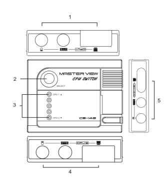
1. CPU Port 1 Connector Ports The extender cables that connect back to the video, keyboard and mouse ports on the computer you are designating as Computer 1 plug in here. Each port is identified by an appropriate icon.
