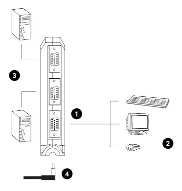
**Note:** 1. In order to fit into the jack, the power adapter cable should have an **L** shaped plug.
