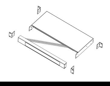
3. Screw the mounting brackets to the rack.
