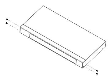
2. Screw the rack mounting brackets into the front and rear modules:
