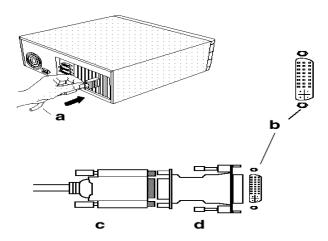
VGA connector from С Display cable а monitor b DVI-I connector on card VGA to DVI- I adapter
