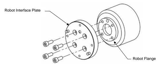
**NOTE:** A Robot Interface Plate is required. The Robot Interface Plate can be purchased from ATI or manufactured by the customer using ATI approved drawings. The use of Robot Interface Plates supplied by ATI is strongly recommended.
