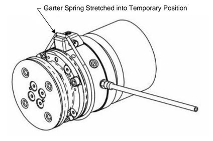
1.6 Slide (1) Coolant Sealant Boot over the Stem Side Interface Plate onto the CPD Cover
