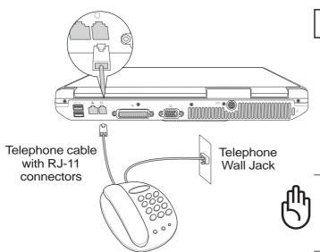
This is an example of the Notebook PC connected to a telephone jack for use with the built-in modem.
