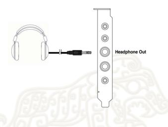
The Headphone Out port has a built-in high-quality amplifier for headphones. Connect your stereo headphones to the headphone output ports on the Xonar Essence ST card.
