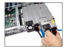
Firmly push the new power supply module into the chassis until the latch locks to the server chassis.
