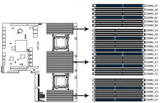
Z9PP-D24 240-pin DDR3 DIMM sockets
