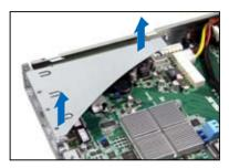
Place the riser card bracket on a flat and stable surface, then remove the screw from the slot bay.
