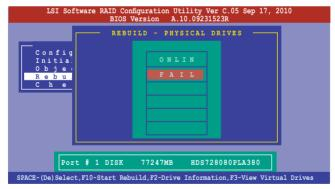
After selecting the drive to rebuild, press <F10>. When prompted, press <Y>
