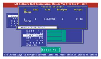
Follow step 10 to 14 of the previous section: Using Easy Configuration to create the RAID set.
