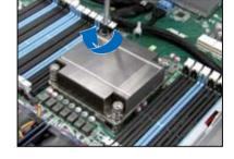
Tighten the four heatsink screws in a diagonal sequence.
