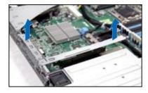
Place the riser card bracket on a flat and stable surface, then remove the screw from the slot bay.
