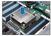
Twist each of the four screws with a Philips (cross) screwdriver just enough to attach the heatsink to the motherboard. When the four screws are attached, tighten them one by one to completely secure the heatsink.
