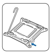
Push down the left load lever (L), and then insert the lever under the retention tab (M).
