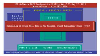
4. When rebuild is complete, press any key to continue.
