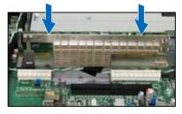
5. Secure the RAID card with the screw that you removed earlier.
