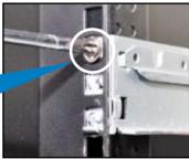
7. When mounting the server to the rack, ensure to include the side knots on the two sides of the server in the rack rail holders, as shown in the right figure.
