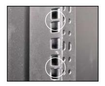
4. From inside the rack, place the rear rail hook on the bottom thin lip of the rear mounting hole, and then place the front rail hook on the bottom thin lip of the front mounting hole, as shown in the right figure.
