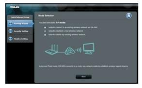
To set up Access Point mode, do not click **Next** on the first page of Quick Internet Setup. Instead, click the link provided to switch setup mode.
