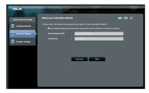
By default, the EA-N66 will assign an SSID using the following format: "original-SSID\_RPT".
