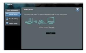
To set up Wireless Range Extender mode, do not click **Next** on the first page of Quick Internet Setup. Instead, click the link provided to switch setup mode.
