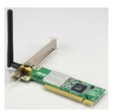
The ASUS WLAN PCI Card (WL-138g) is a wireless LAN adapter that fits into a standard PCI slot in a desktop PC and creates a wireless network using the IEEE 802.11g/b wireless standards.
