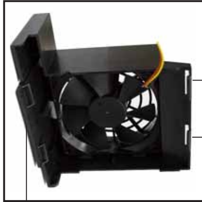
Outer side of fan cage Side tabs Inner edge of drive cage
