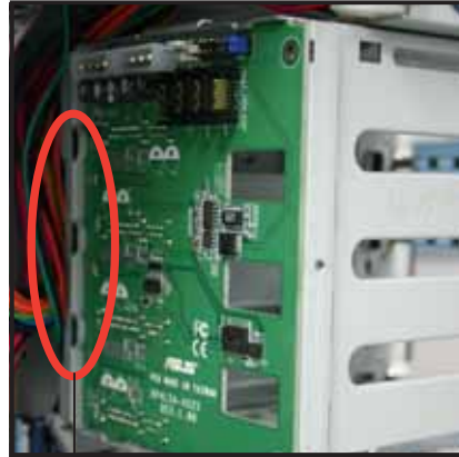
Outer side of fan cage Side tabs Inner edge of drive cage
