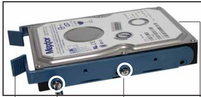
Rail handle Hole 1 Hole 3 Drive connectors
