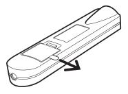
Move the on/off button on the right side of the remote control to the "on" position by sliding it up. To confirm that it is on, push the small round button located right above the Atek logo to see if the white LED illumination light below the logo turns on.
