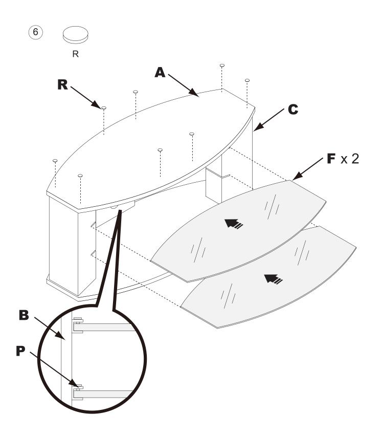
6, Place glass shelves(F) through slot in side columns (C) until they stop at back board (B) and rest in glass supporter (P). Place the glass protector (R) on the top board (A).
