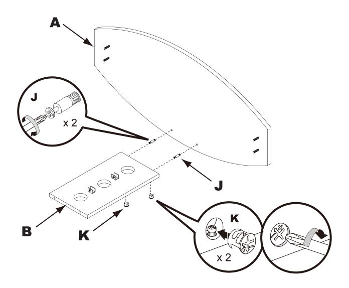
2. Attach back board (B) to the top boards (A) with screws (J), and cam locks(K). Turn cam lock(K) clockwise to secure.
