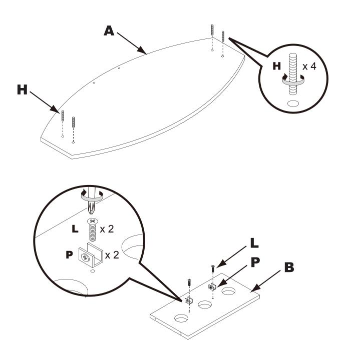
1. Fasten screw (H) to the top board (A). Fasten glass supporter (P) to the back board (B) with screw (L).
