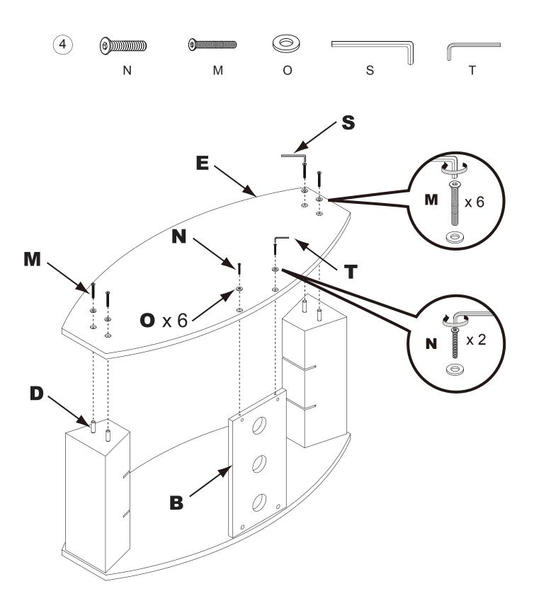
4. Fasten bottom board (E) to the tube (D) with screw (M) and washer (O), then secure to the back board (B) with screw (N) and washer(O).
