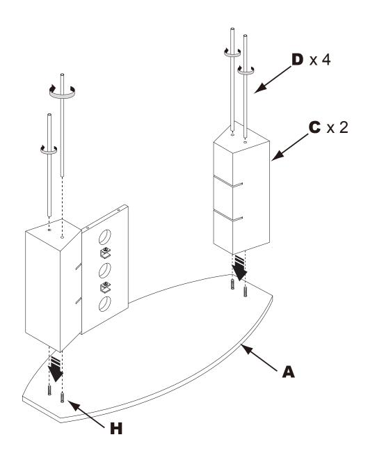
3. Fasten tube (D) to the top board (A) with screw (H) and turn clockwise to secure. Then put the side column (C) on the top board (A).Insert tubes(D)through side colums(C) and rotate clockwise to secure.
