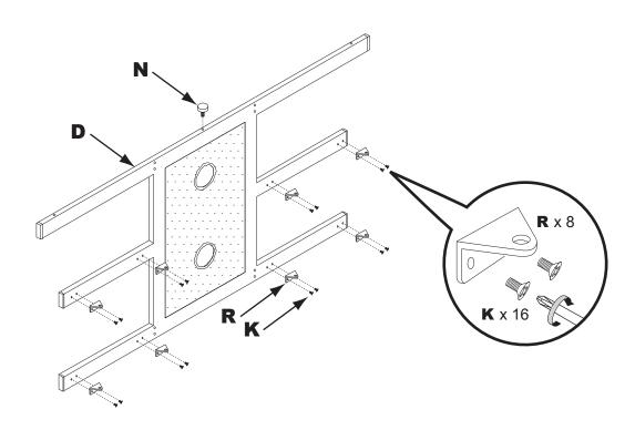
2-Fasten glass supporter (R) to the frames (D) with screws (K). Fasten glass protector (N) to the frames (D) .
