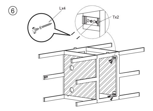
6-Fix the parts of hinge(T) to side board(F) with screws (L)
