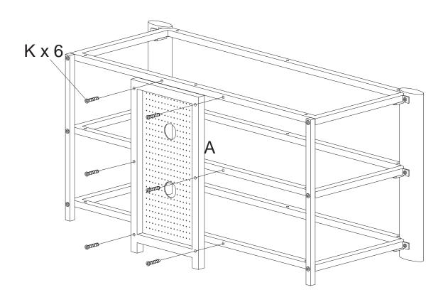
3. Attach back panel (A) to the unit with screws (K).
