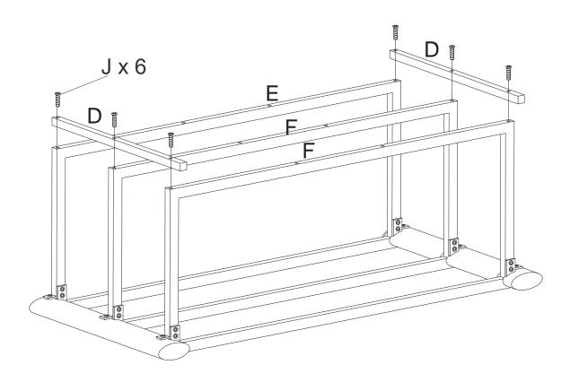
2. Fasten pillars (D) to the frames (E&F) with screws (J)
