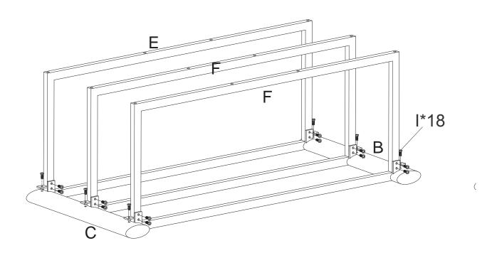
1. Attach frames (E&F) to the pillars (B&C) with screws (I).
