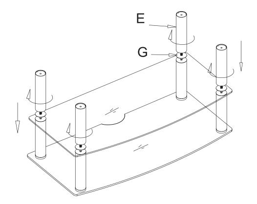
3. Put the rubber pads (G) on glass (C), then screw pillars (E) on the glass (C).
