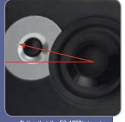
Notice that the FS-4000's tweeters are offset above the centerline of the woofers. This is a perfect example of the way that Atlantic pays close attention to acoustic details. By moving the tweeters up, we significantly reduce the audibly-intrusive interference patterns that result from woofers and tweeters being mounted side-by-side.
