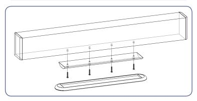
5. Using Atlantic's exclusive center channel rocker base, the FS-4000 can be used as a freestanding speaker on a TV or on a shelf in addition to wall mounting.
