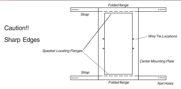
This kit is intended for use only with the Atlantic Technology IWTS-10 InWall speaker. It is intended to be used in new construction where a "place holder" is needed for the wall board or plaster contractor to locate an appropriate opening for the speaker.
