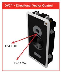
By flipping the DVC switch to "on," we electronically manipulate the crossover so that the speaker's midrange output lobes down about 15 degrees from the speaker. This is perfect for when this speaker is mounted above ear level and you want to
