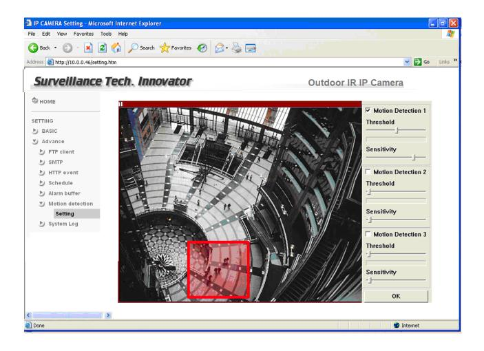
Click it **On** when you use the Motion Detection function and detecting zone appears for adjusting and moving. The common setting options are displayed below. If you do not wish to use the Motion Detection function, click it **Off** and press **OK**.
