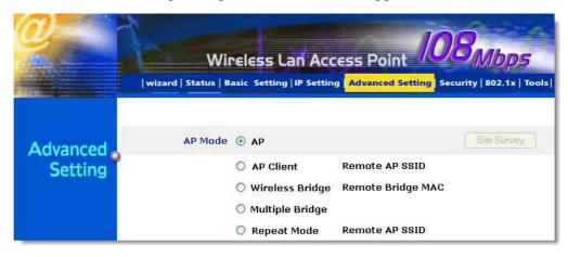
**1 AP:** The normal Access Point operating mode which forms a wireless ESS network with its wireless clients. In figure an example of configuration.
