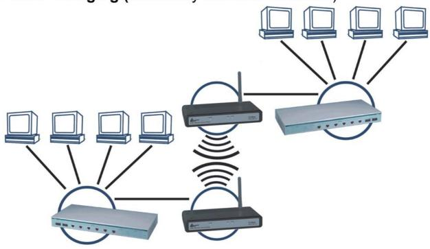
**4 Multiple Bridge:** A group of APs which consists of two or more APs operating under Multiple Bridge mode, that can connect two or more Ethernet networks or Ethernet enabled clients together. All APs have to use the same **Channel** and **SSID** in order to set a Multiple Bridge network.
