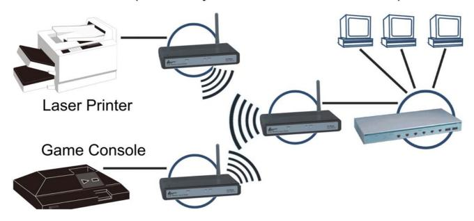
**3 Wireless Bridge:** A pair of APs operating under Bridge mode to act as the bridge that connect two Ethernet networks or Ethernet enabled clients together. You must make sure that the SSID and Channel is set the same as that AP you wish to connect. **Remote Bridge MAC filed**: key in the **LAN Mac address** (NOT wireless Mac address) of the AP that you wish to get connected.
