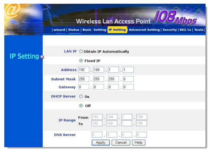
The default IP address of this access point is **192.168.1.1** with the subnet mask of **255.255.255.0**. You can type in other values for IP Address, Subnet Mask and Gateway and click "**Apply**" button for the changes to be effective.
