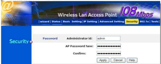
**Password:** Allow you to change the new login password. Here are the necessary steps: 1. Enter the new password in the "AP Password New:" field. 2. Enter the new password again in the "Confirm" field. 3. Click "Apply"
