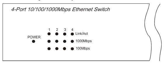
The 4-port 10/100/1000Mbps Gigabit Ethernet Switch LED indicators
