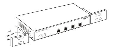
Attaching the mounting brackets to the Switch
