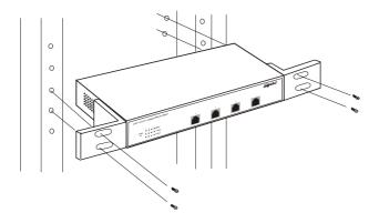
Installing the Switch in an equipment rack
