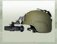
The NVM14-2 is a high performance, versatile night vision monocular. It is designed to be multifunctional: hand-held as a monocular, head-mounted/ helmet-mounted as a single-eye goggle, or weapon- mounted as a night scope.
