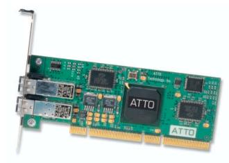
Dual-channel, Low-profile 2-Gigabit Fibre Channel Host Adapter provides compact design and high performance
