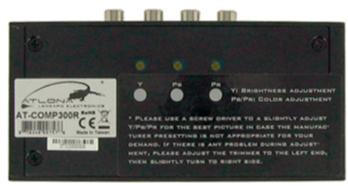
\* Please use a screw driver to a slightly adjust Y/Pb/Pr for the best picture in case the manufacturer presetting is not appropriate for your demand. If there is any problem during adjustment, please adjust the trimmer to the left end, then slightly turn to right side.
