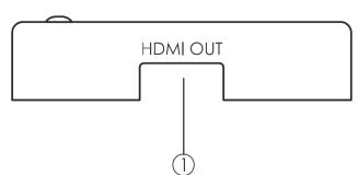
1. HDMI OUT: This slot is where you connect to a HDTV display with a HDMI cable for source signal display.
