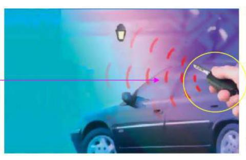
Encoder + Transmitter RF UHF in the key
