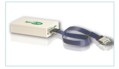
The SuperTrace<sup>™</sup> Probe, Green Hills<sup>®</sup> Probe and Slingshot<sup>™</sup> debug device are advanced hardware debug devices that enable the MULTI<sup>®</sup> integrated development environment to load, control, debug and test a target system without the need for prior board initialization, an RTOS, or even a ROM monitor.
