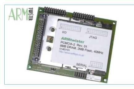
The **ARMtwister** is a small embedded control board with PCMCIA socket utilizing the Atmel AT91M40800 Microcontroller. With its customized version of uClinux-2.4 it is possible to use IEEE 802.11 Wireless PCMCIA cards, as well as Ethernet cards and most other 16-bit PCMCIA cards.
