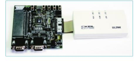
The Keil ULINK USB-JTAG Interface Adapter connects the USB port of your PC directly to the JTAG port of Atmel AT91 ARM devices. Using the  $\mu$ Vision Debugger with ULINK, you can easily create, download, and test embedded applications on actual target hardware.
