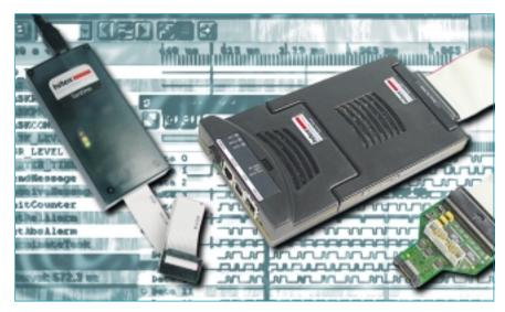
**Tantino for ARM7-9** is our compact and cost-effective USB-to-JTAG debug interface. It supports all run-control debug facilities like breakpoints, watchpoints, single-step, register and memory view. Together with the HiTOP IDE, you have everything to compile and debug your application including RTOS support.
