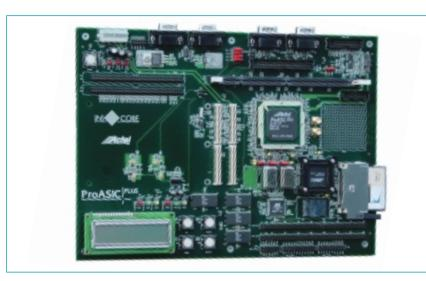
The **SDB-750/1000** is powered by the ARM7TDMI 32-bit RISC processor based AT91R40807. In combination with the 2 Mbytes SRAM and 16 MBytes of program memory (FLASH), the board operates in a standalone mode. It is available with an up to one million gates ProASIC PLUS FPGA from Actel.
