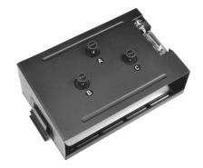
In the large opening of the Atomic Amp, you will see three round cavities, like circles in a cornfield. This is where the mushroom heads of the locking screws fit.
