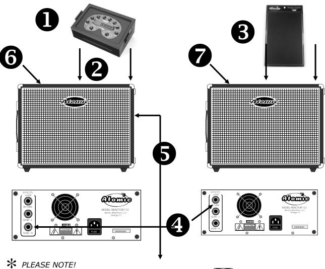
If you wish to use a pair of Reactors in MONO, simply use the SEND – L output instead of SEND – R.
