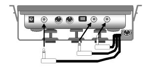
Use the power cable included with the docking template to connect between your modeler's power input and the DS-1s power output. THERE IS NO NEED FOR AN EXTERNAL POWER SUPPLY.
