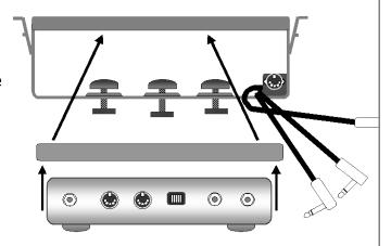
After securing modeler, connect the Input and, Left/Right output connectors. The Input cable is extra long to accommodate modelers that have their input jacks located on the front. Please note that there is plenty of room to get to foot controller connections etc. If your modeler has a ON/OFF switch, switch it ON now.
